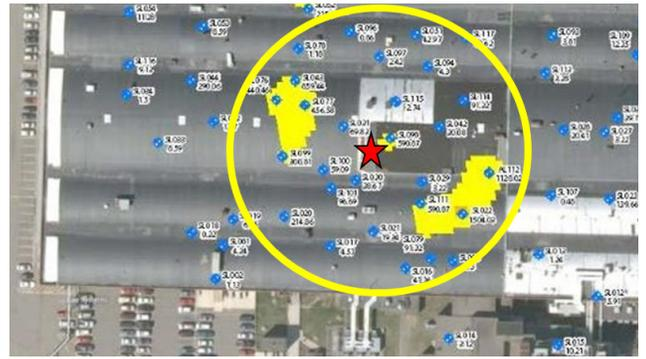
One HVS test (red star showing suction point and yellow circle showing radius of influence) can replace multiple traditional sub-slab soil gas samples (blue dots).
